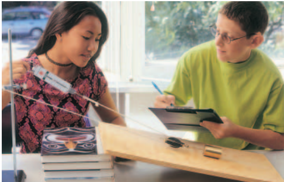
Figure 2.8 The measured mechanical advantage of this system was less than the speed ratio when the students tested it.
