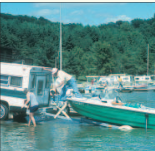
Figure 2.7 The ramp is an inclined plane that helps to lift the boat onto the trailer. The winch is a wheel and axle with a cable on it. It pulls the boat up the ramp and onto the trailer.
