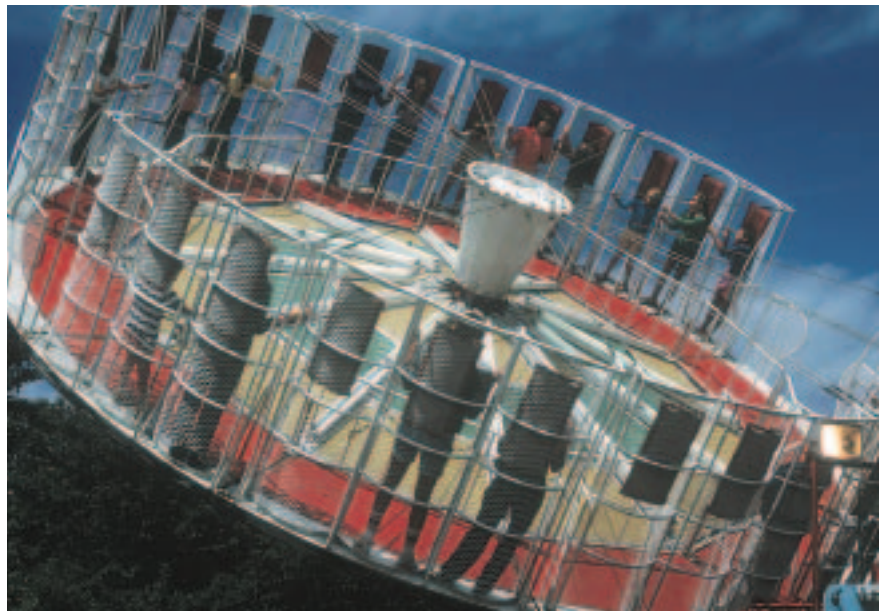
Figure 2.20 This ride uses a hydraulic system to create thrills. Hydraulics in the base of the ride lift and slant the platform as it spins.
