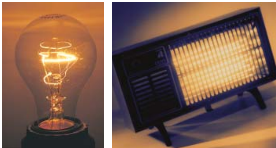
Figure 2.5 The tungsten filament in an incandescent bulb and the element in a heater both radiate heat and light because of resistance.
