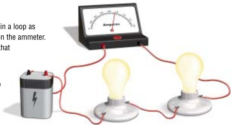
Figure 2.17 This ammeter will read the current for the circuit. The circuit shown has only one pathway, so the current is the same everywhere in the circuit.
